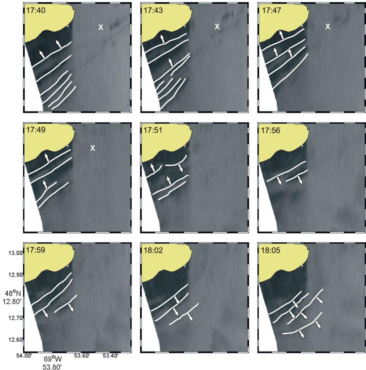
FIG. 9. Sequence of georectified photographs showing the wave train progression as it collided and reflected off the southern flank of PC. Vectors only indicate propagation direction. The time is in UTC.
