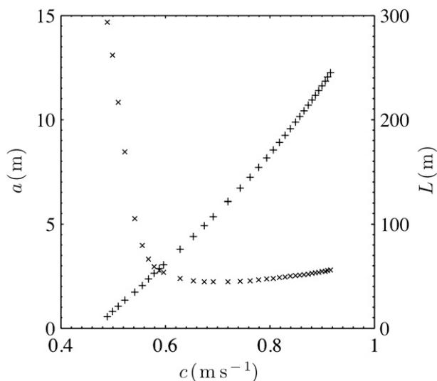
FIG. 12. Theoretical relationship between amplitude  $a$  (denoted by plus symbols), wave horizontal length scale  $L$  (denoted by crisscrosses), and wave phase speed  $c$ . These functions are used to infer wave amplitude and length scale from the phase speed measurements.
