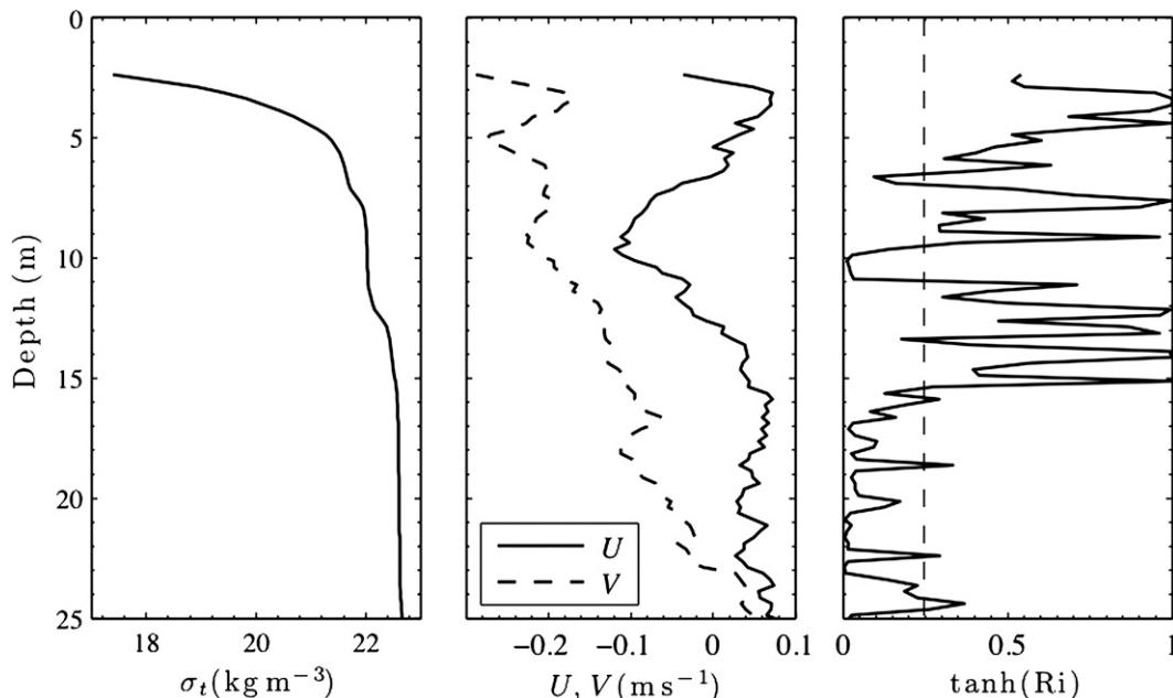
FIG. 8. Background conditions off PC prior to the passage of the wave train of Fig. 4: (left) 1-m-scale density profile just ahead of the leading wave (profile 1 in Figs. 4, 5); (middle) 1-m-scale and 60-s-average across-wave ( $U$ ) and along-wave ( $V$ ) current; and (right) 1-m-scale Richardson number with the dashed line located at the critical value  $Ri_c = 1/4$ .
