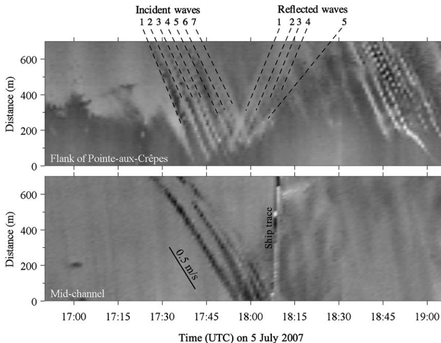
FIG. 6. Internal wave rays seen from a space-time representation of the georectified photographs interpolated along (top) an axis extending off the southern flank of PC and (bottom) a midchannel axis (see Fig. 3). The numbered dashed lines in (top) are visual aids to help identify incoming and reflected wave rays.
