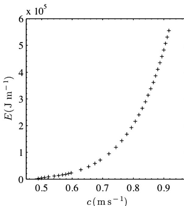
FIG. 13. Theoretical relationship between wave mechanical energy  $E$  and phase speed  $c$ .
