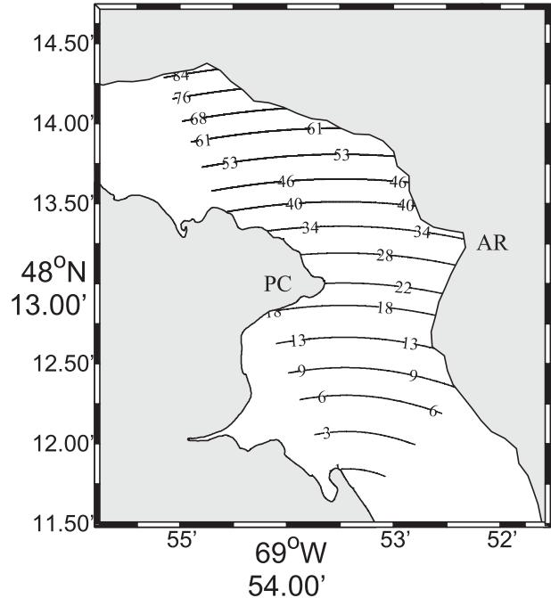
FIG. 2. Effective pixel resolution  $\Delta$  (m) of the georectified images. Phase speed measurements presented in section 3 (see Fig. 6 and Tables 1, 2) were taken from the southern flank of PC, where the resolution is  $13 \text{ m} < \Delta < 18 \text{ m}$ . This is about  $1/3$  of inferred wave horizontal length scales  $L$  (see Table 1).
