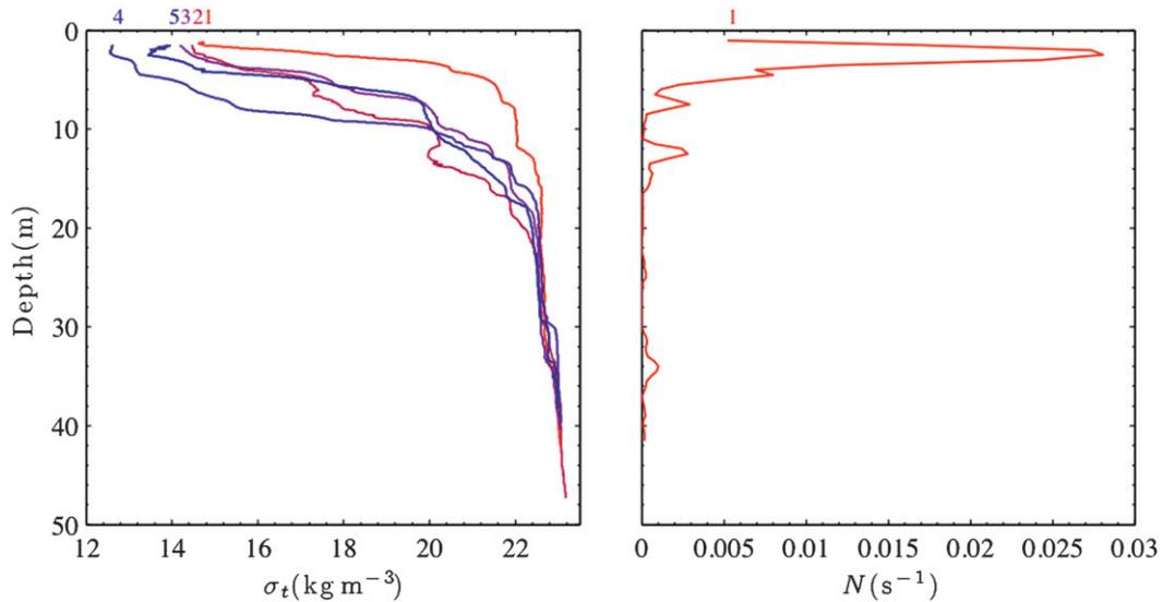
FIG. 5. (left) Density profiles collected through the wave train of Fig. 4 and (right) 0.5-m scale buoyancy frequency  $N$  of profile 1. The pycnocline is located at depth  $h_1 = 2.5$  m and is characterized with  $N = 0.028 \text{ s}^{-1}$ . The color-coded numbers 1–5 above the figure are identification labels for comparison with Fig. 4.
