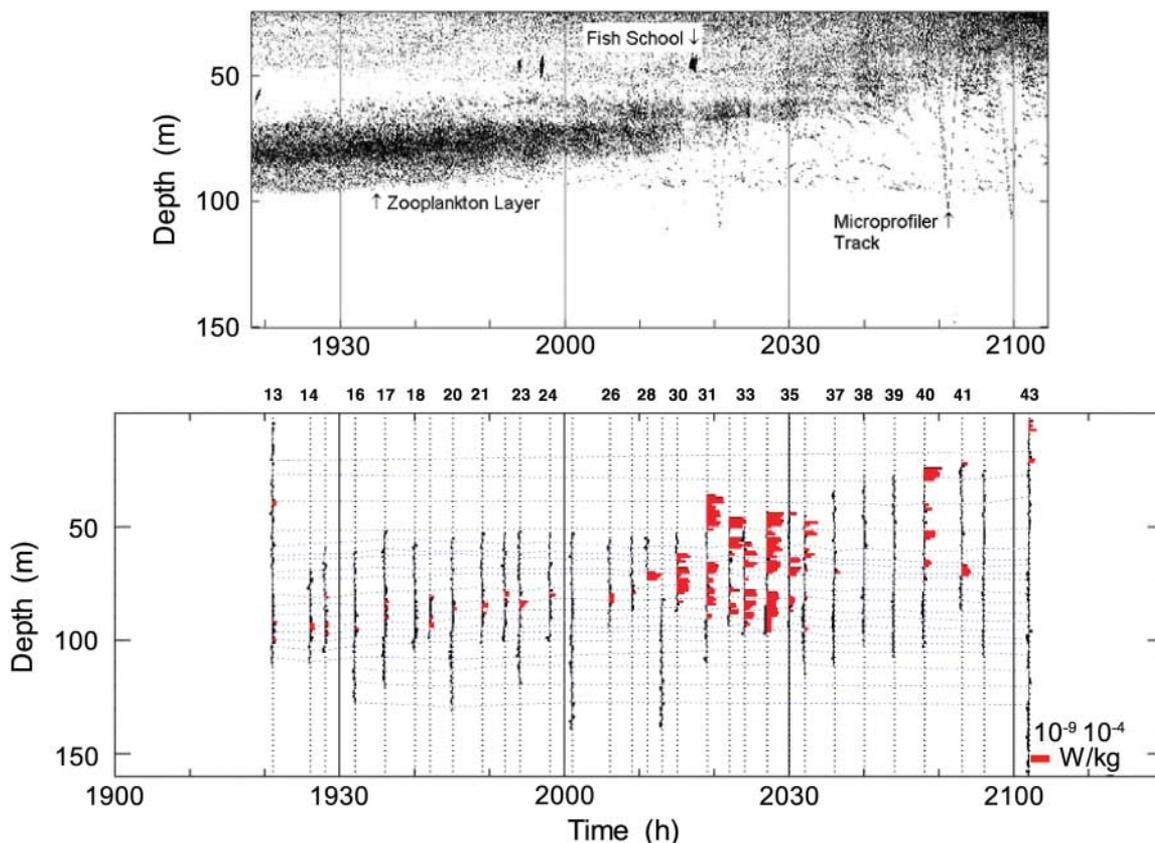
by previous microstructure measurements. Despite its short duration, this episode was sufficient to boost daily-averaged turbulent eddy diffusivities in Saanich Inlet by two to three orders of magnitude. Daily-averaged diffusivities are  $0.02 \times 10^{-4} \text{ m}^2 \text{ s}^{-1}$  when dusk and dawn enhancement are excluded but  $4 \times 10^{-4} \text{ m}^2 \text{ s}^{-1}$  to  $40 \times 10^{-4} \text{ m}^2 \text{ s}^{-1}$  when they are included.
