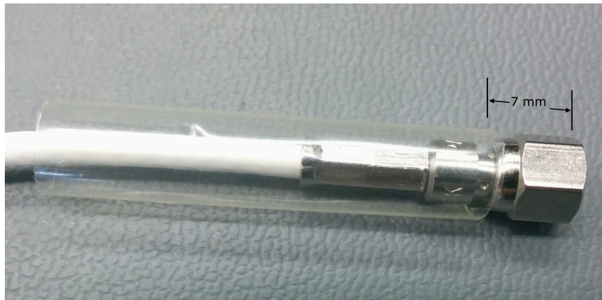
Figure 3: The heat shrink tubing covering the shaft of the SMC cable before heat has been applied. The heat shrink is positioned 7 mm behind the front of the nut.
