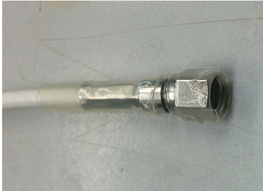
Figure 1: SMC cable with damaged heat-shrink tubing.
