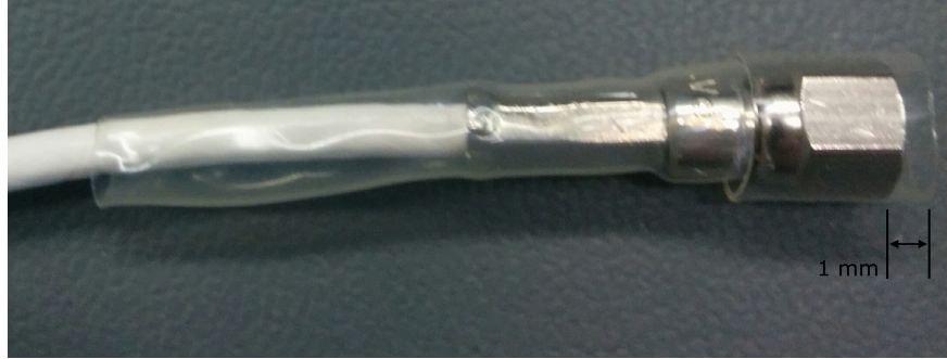
Figure 4: Tubing on shaft, partially heated, and new tubing on nut before heating.
