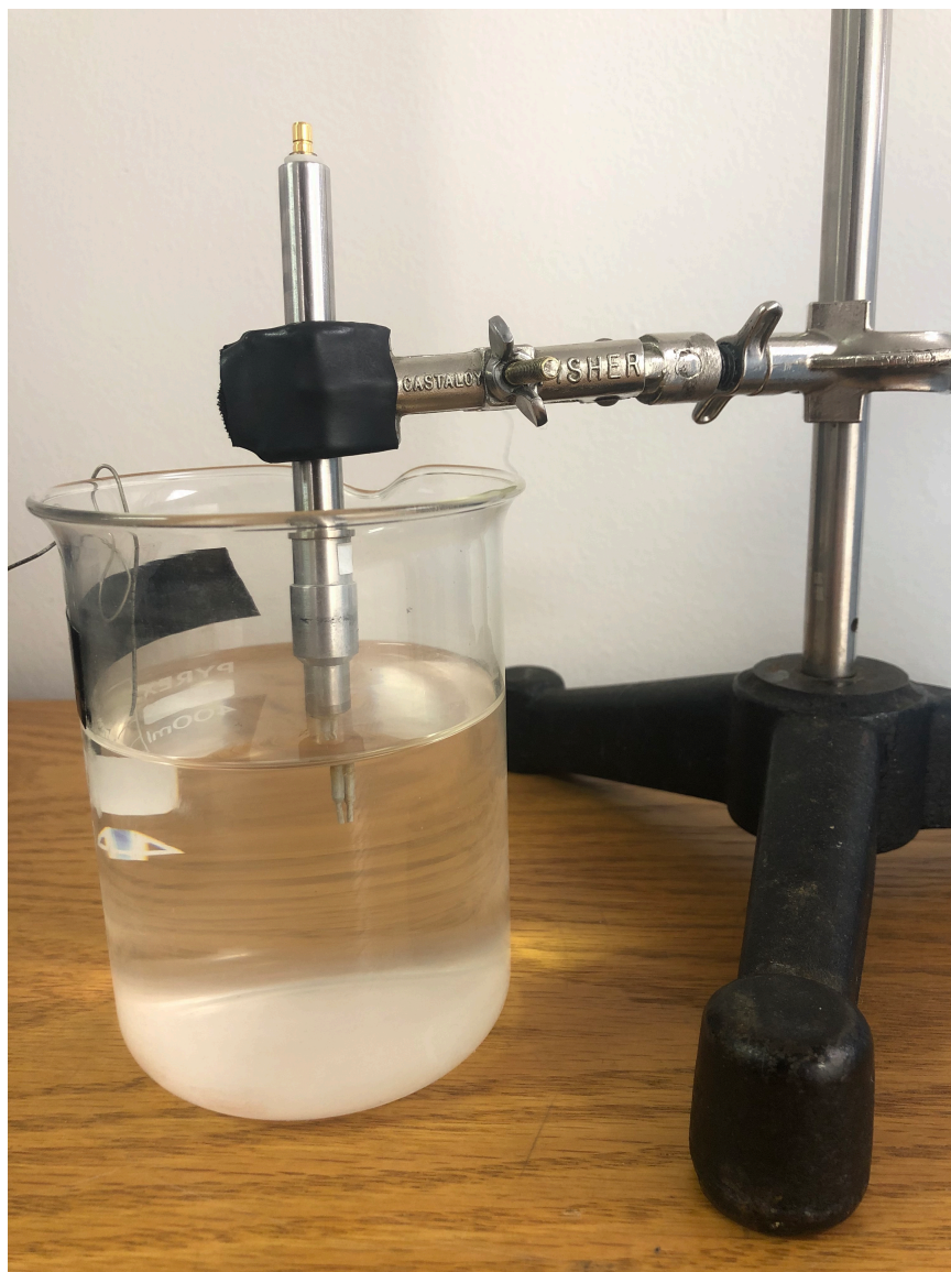
Figure 1: A SBE7 Micro-conductivity probe soaking in Triton X-100 solution. A magnetic stirrer may need to be added for improved effectiveness.
